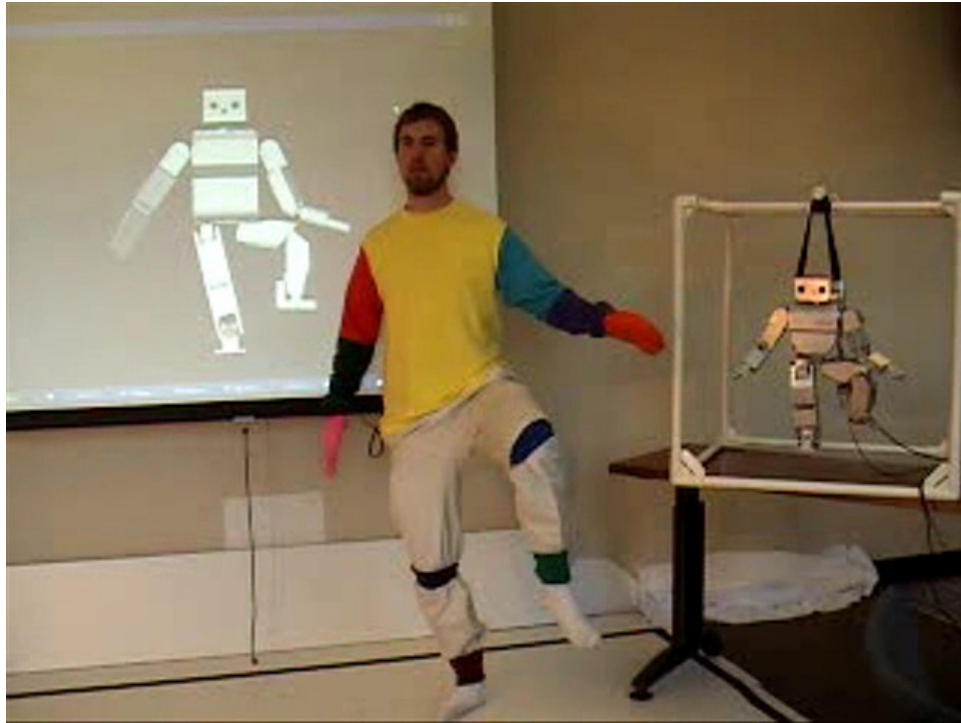
Figure 5.1: Setup for a full system demonstration of real-time imitation using the HOAP-2 humanoid robot.
